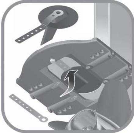
**Determine the final position of the SE Sport Hydrofoil** by resting it on the **Top Clip** of the Sport Clip. *The four holes in the Hydrofoil will align fully with the Top Clip when installation is complete.*
